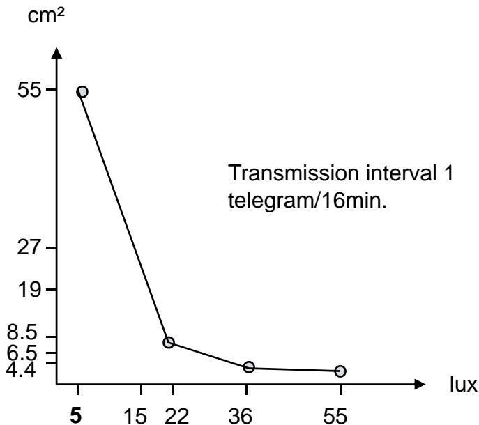
The graphic shows the required minimum luminous intensity (in lux) for operational readiness of the STM100, dependent on differently sized solar generators.
