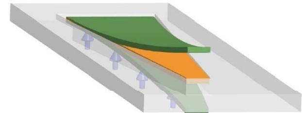
Fluidic oscillator for generation of oscillations
